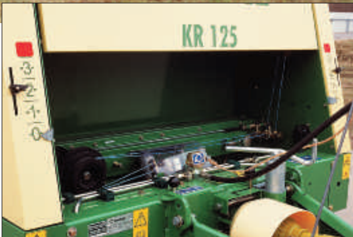
Keep in shape: pressure indicators on either side of the frame show the evenness of fill in the bale chamber making the operator's life easy. The baler can thus be filled uniformly over its entire width, that means top quality bales!
