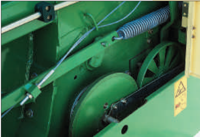
Get wrapping: the net wrap is fed into the bale chamber by one rubber coated roller pressing against a fixed aluminium roller. The lateral friction wheel initially drives the rollers with the number of net wraps infinitely variable and set via the threaded rod.
