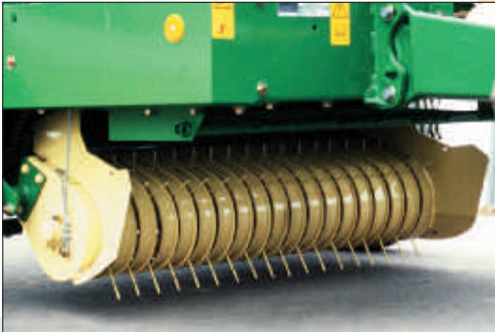
The KR 125 pick-up has a clearing width of 1400 mm (55") (DIN 11220). Hydraulically raised and lowered it is quickly and easily set to the desired height. The short feed path from pick-up to bale chamber ensures a continuous crop flow.
