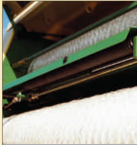
Hydraulic starter: With this option a hydraulic cylinder initiates the binding process. The hydraulic starter is operated via the tractor spool valve or the control panel of the Comfort Kit option.
